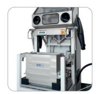
The Part Removal Station PRS is a basic feature of the SLM 500. This useful component of the machine is optimally suited for batch production, and serves for removing the excess powder from the build cylinder and the build parts.
