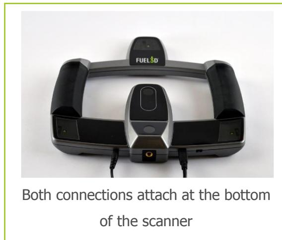
Select the appropriate power adaptor for your region. Plug the power adaptor into a power outlet and the other end into the scanner. Plug the USB into the scanner and your PC.
