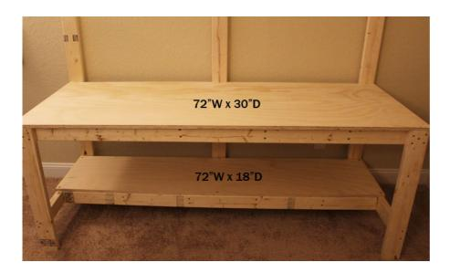
After the horizontal pieces of plywood are secured, go ahead and attach the back panels to the frame.
