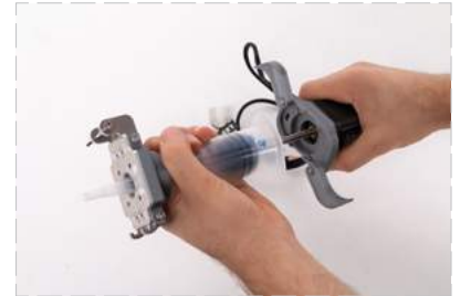
Pull the piston out from the syringe.
