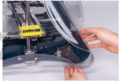
Pull out the cover rear corner from the machine frame.
