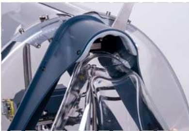
Pull out the cover upper corner from the machine frame.
