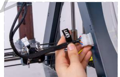
Connect the 'LEFT' connector to the Left socket on the machine frame.
