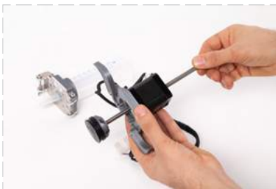
Manually move the piston to the starting position.
