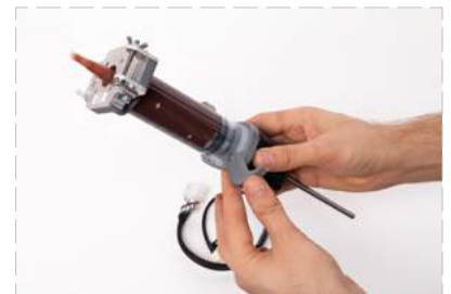
Push the piston inside the syringe and lock the syringe blockade.
