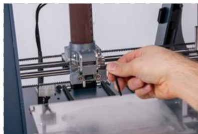
Screw tight the front screw.
