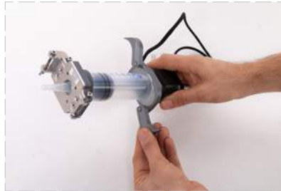
Unlock the syringe blockade.
