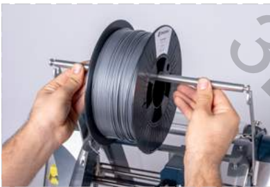
Loosen the screws to the point where you can slide the spool holder.
