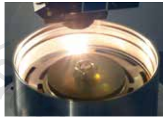
Laser welding the housing of a water pump clutch.
