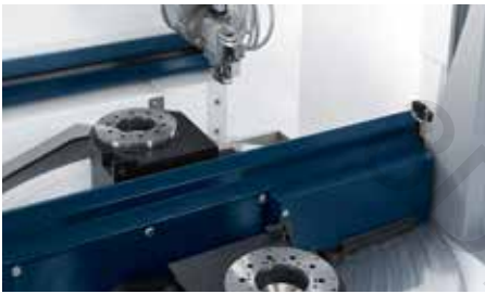
Rotary changer with rotating axis.
