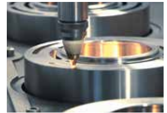
Laser cutting the housing of a water pump clutch.
