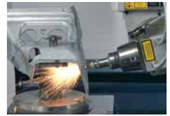
Laser cutting a seatbelt panel.
