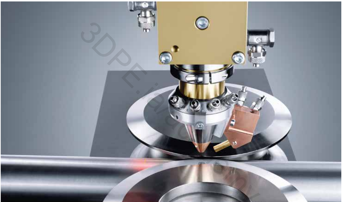
Continuous welding of tubes.
