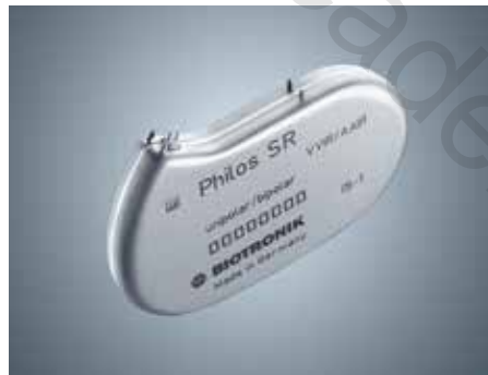
Seam welding temperature-sensitive components, such as titanium pacemakers.
