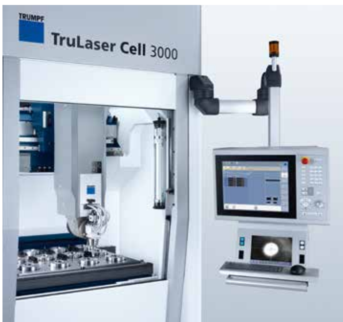
Laser cutting with customized fixture technology.
