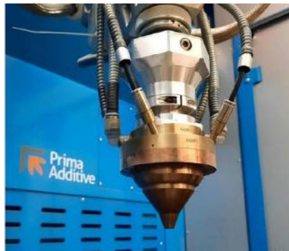
High Precision Configuration Thin spot to create thin features with superior surface quality
