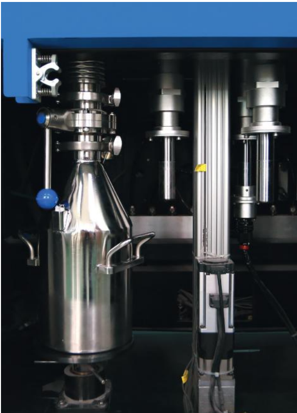
Automatic collection of excess powder not deposited during the process
