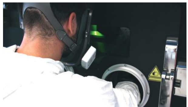
Safe powder management through a glovebox access door
