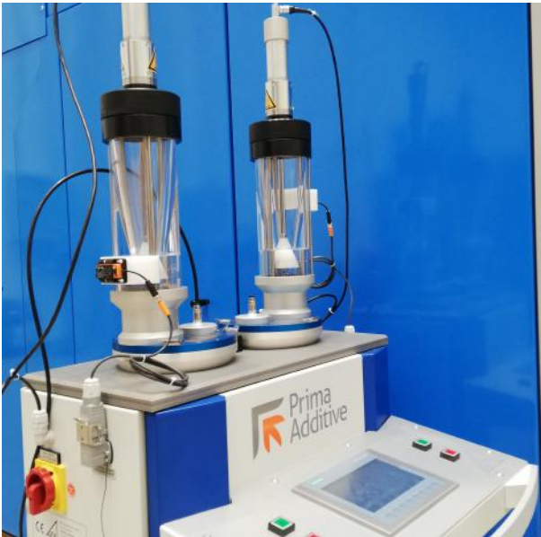
A modular powder feeder suitable for rapid change of material processed or for back-up
