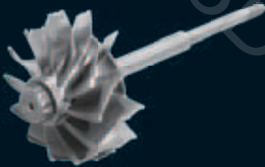
Repair of turbo impeller for large diesel engine - Inconel 713 parent material - Inconel 718 deposition material
