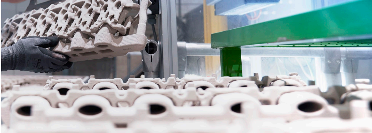
The German automaker BMW Group uses sand binder jet systems from Desktop Metal's ExOne brand with sustainable inorganic binder for production 3D printing of the sand cores needed to metalcast water core jackets for automotive engines. The use case of sand binder jetting is a blueprint for the future of metal binder jetting technology for production.
