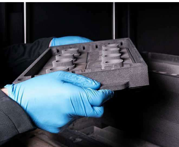
After curing, parts are depowdered, as shown above. Finally, parts are sintered in a furnace where powder particles fuse into a high-density part that typically exceeds a gravity casting and meets or exceeds standard MIM parts.
