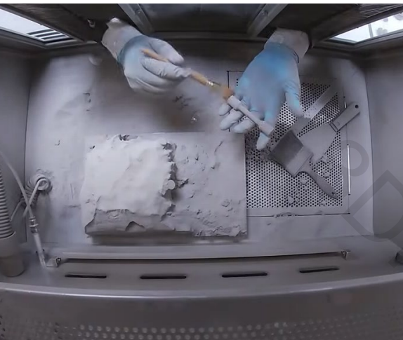
After curing, parts are depowdered, as shown above. Finally, parts are sintered in a furnace where powder particles fuse into a high-density part that typically exceeds a gravity casting and meets or exceeds standard MIM parts.
