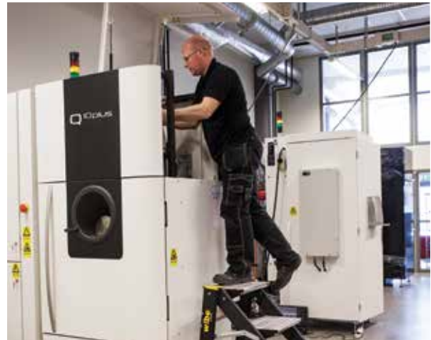
Field Service engineer performing scheduled maintenance.
