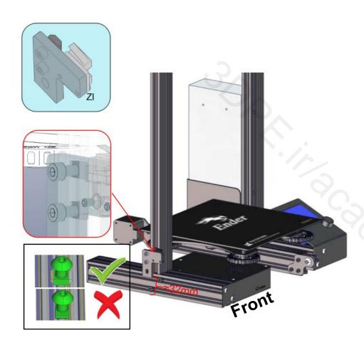
1. Prepare limit switch assembly (ZI) and 3mm Allen key;
