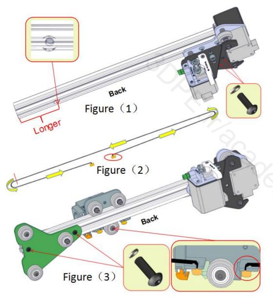
Step 1. Assembly of aluminum profile (B1) and extrusion assembly (E). Aluminum profile (B1) is shown in the diagram on the left(1). Pay attention to the position and direction of the large hole. Align the hole of extrusion assembly (E) with the threaded hole of aluminum profile (B1), it should be noted that the hole has two plates, which aresecured with M4\*16 screws, and fixed to the second profile plate and the aluminum profile (B1). Use a suitable Allen key to tighten the screws.
