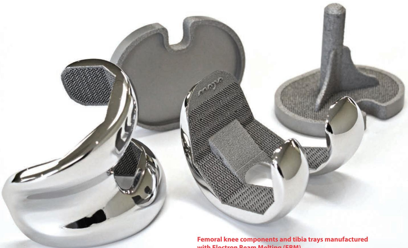
**Femoral knee components and tibia trays manufactured with Electron Beam Melting (EBM).**
