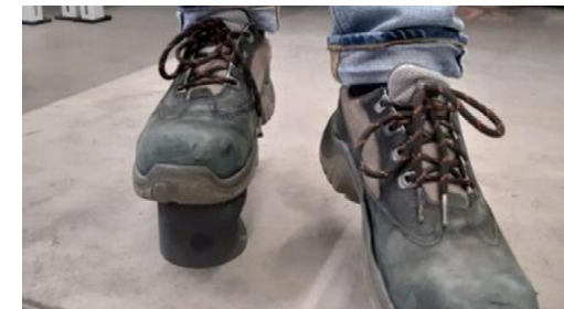
Stress test for a green part made of heavy metal alloy
