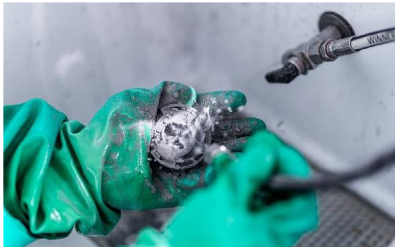
Depowdering with water jet
