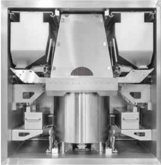
Arcam Q20plus build chamber.
